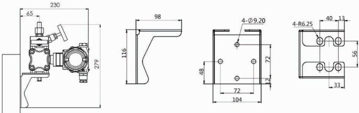
BRACKET DE MONTAJE EN I (B3) (MEDIDAS EN MILÍMETROS).
