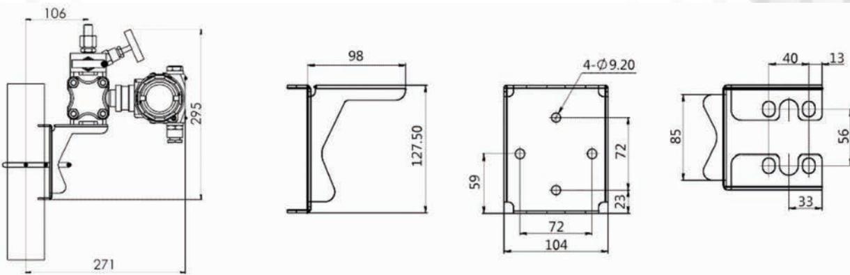
BRACKET DE MONTAJE COPLANAR (B2) (MEDIDAS EN MILÍMETROS).
